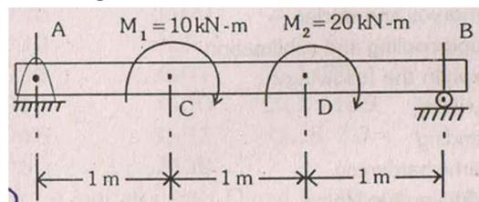
Find the ratio of deflections in the beam at locations C and D where the couples are acting.
