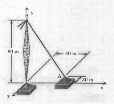
A tower guy wire is anchored by means of a bolt at A. If the magnitude of the tension in the wire is 2500 N, determine the components of the force acting on the bolt in the x, y and z directions.
