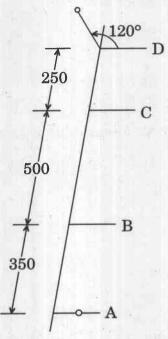
A rotor is completely balanced when masses of 2 kg and 1.2 kg are added temporarily in planes A and D each at 200 mm radius as shown in the figure. The balanced mass in the plane A is along the x-axis whereas in the plane D, it is at 120 mm radius. Determine the magnitudes and the directions of the masses B and C.
